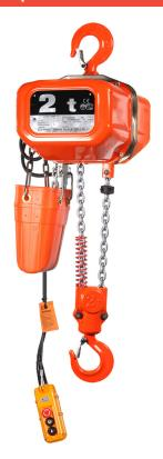
The 400 V electric chain hoists are extremely solid and have a robust sheet steel housing. Very popular as it is ready to use with limit switches, 24 V control voltage, controlunit and plug connections. The high duty cycle and high lifting speed ensure trouble-free operation and a long service life.
